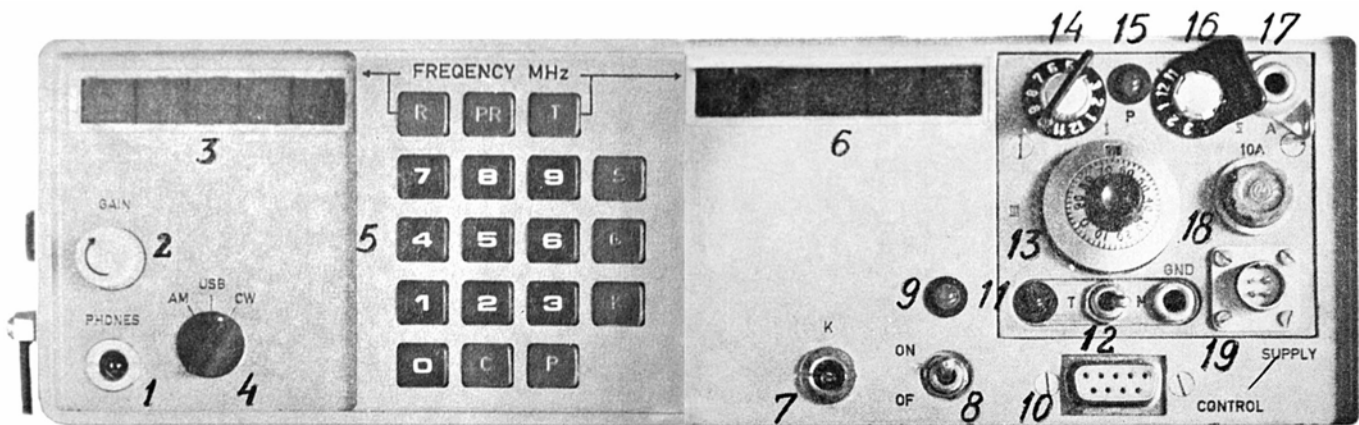
Explanation of controls M-135P: 1= Earphone socket, 2= AF gain control, 3= Receiver frequency display, 4= Receiver operating mode switch, 5= Frequency entry keyboard, 6= Transmitter frequency display, 7= Morse key socket, 8= On/off switch, 9= System 'on' indication led, 10= High speed Morse keyer input, 11= TX 'on' led, 12= Transmit/receive switch, 13-16= Aerial matching controls, 17= Aerial socket, 18= Fuse, 19= 12V DC input.
